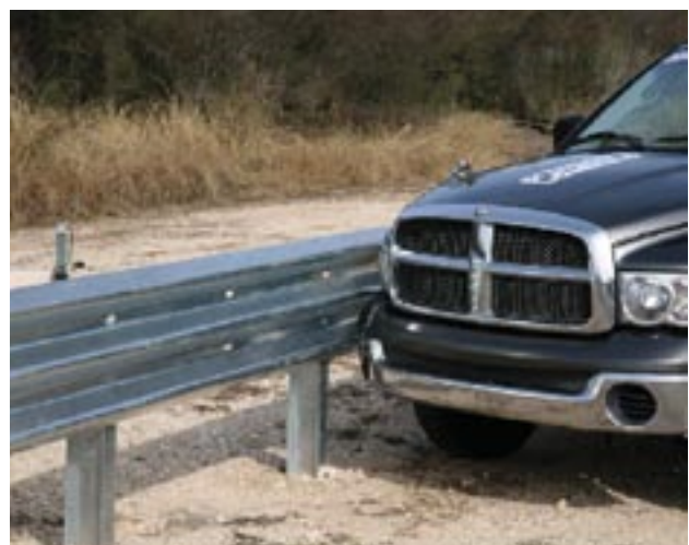
2270kg pick-up truck - 100km/h and 25° (TL3 impact)
