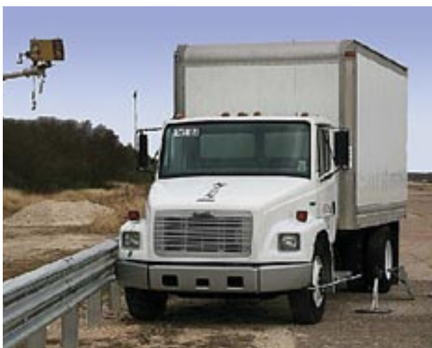
8000kg single unit truck - 80km/h and 15° (TL4 impact)
